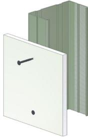
**Plasterboard on Metal** ( up to 0,7 mm metal )
